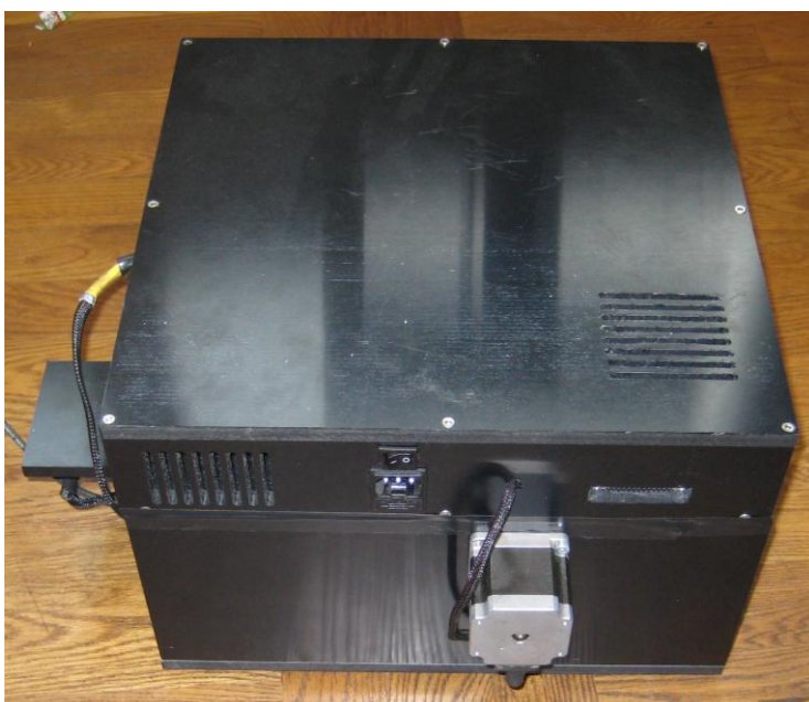
Figure 1. Laser scanner developed for road texture measurements.
