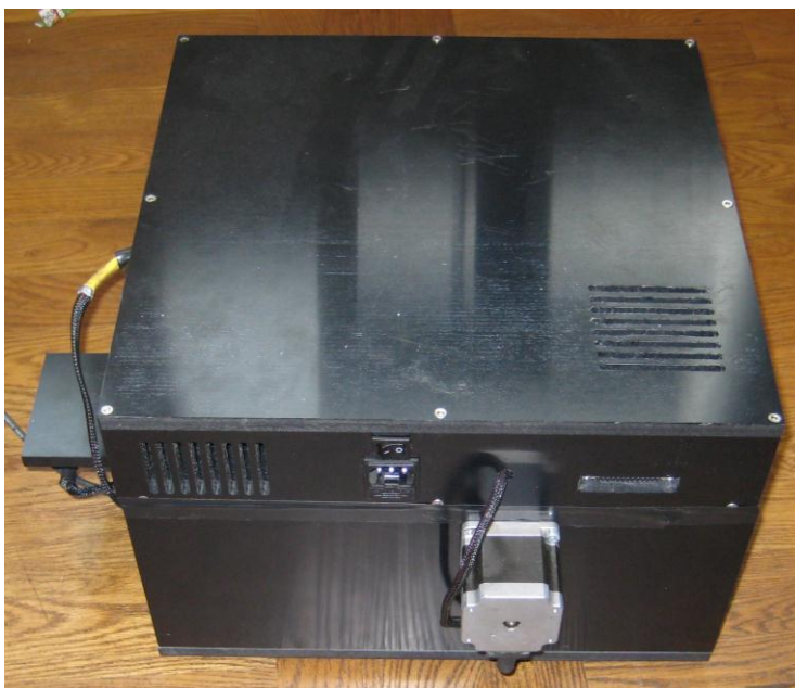
Figure 1. Laser scanner developed for road texture measurements.
